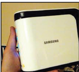
FIGURE 5: Sprint's Airave femtocell – a handheld cell site
